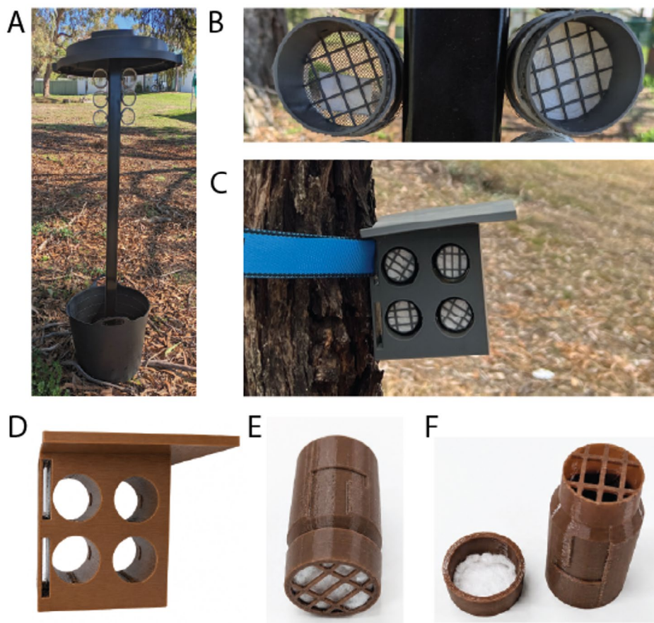
FIGURE 1 | Passive airborne eDNA sampling devices used in this study. We deployed two passive eDNA collection platforms. (A–B) Filter surface area trial platform : (A) full view of the custom-built device constructed from a vertical fence post set in a concrete-filled bucket and fitted with a bin lid for rain protection, with multiple filter holders mounted along the post; (B) close-up of the PVC Mozzie Stoppa trial units with 3D-printed filter holders shown inserted to vertically hold differently-sized filters (2.5 × 2.5 and 5 × 5 cm); (C–F) 3D-printed passive air sampler : (C) field deployment of the platform with a strap securing the unit to a tree; (D) close-up of the housing showing four cartridge insertion points, including the internal locking mechanism to prevent cartridge displacement; (E) assembled filter cartridge showing the recessed channel that engages with the locking mechanism; (F) disassembled filter cartridge illustrating placement of the circular filter within the cartridge cap.
