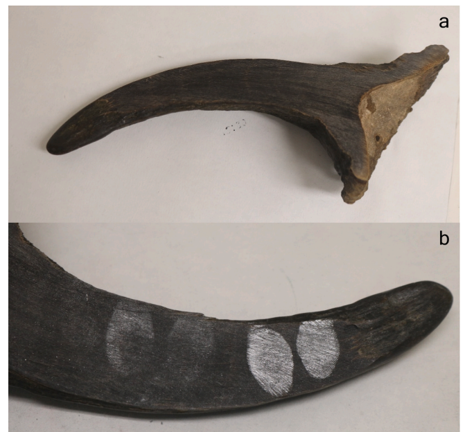
Fig. 1. Pictures displaying one half of the cut rhino horn that was used throughout these experiments with no fingermark enhancement (a) and fingermarks visualised with aluminium powder on the interior surface of the cut rhino horn (b).
