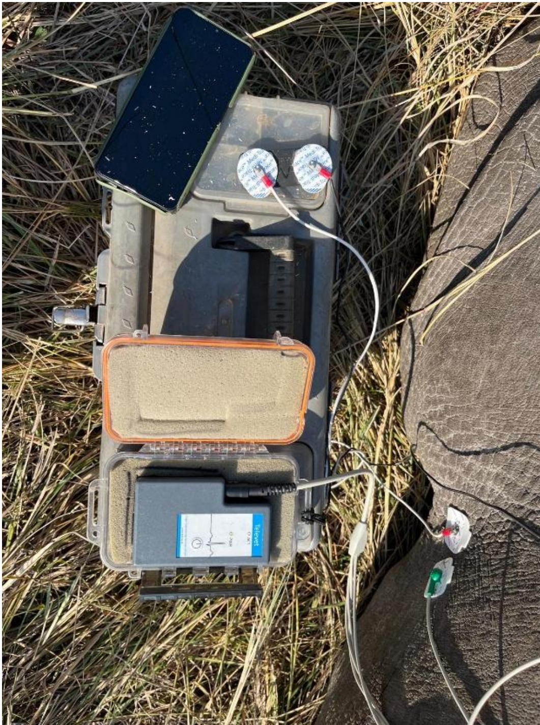
Figure 1. Modified KardiaMobile (upper device) and Televet 100 (lower device) are shown in research setting. Photo by author.
