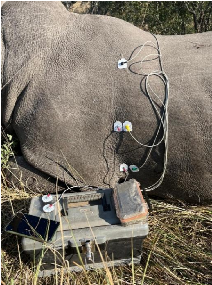
Figure 2. Electrode placement on left side of the thorax of a white rhinoceros ( Ceratotherium simum ). The modified KardiaMobile is shown left on top of the box. A white cable connects to the lower electrode on the rhinoceros and a black cable to the upper electrode. Right on top of the box the Televet 100 is shown inside its protective case. Green, yellow, and black connections attach to the lower, middle, and upper electrodes respectively. Photo by author.
