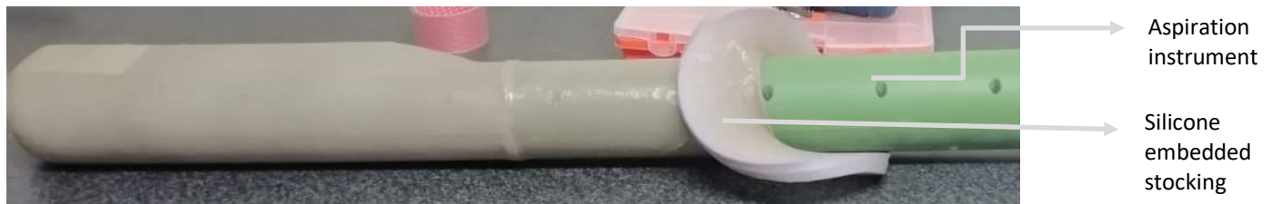
Figure 4: An in vitro temperature simulation study was conducted to ascertain whether the measured outside temperature of the aspiration instrument (used to recover oocytes during transrectal ovum pick-up in southern white rhinoceros) was an accurate indication of the inside temperature, the aspiration instrument was encased in a silicone-saturated elastic stocking to simulate the rhinoceros rectal membrane.
