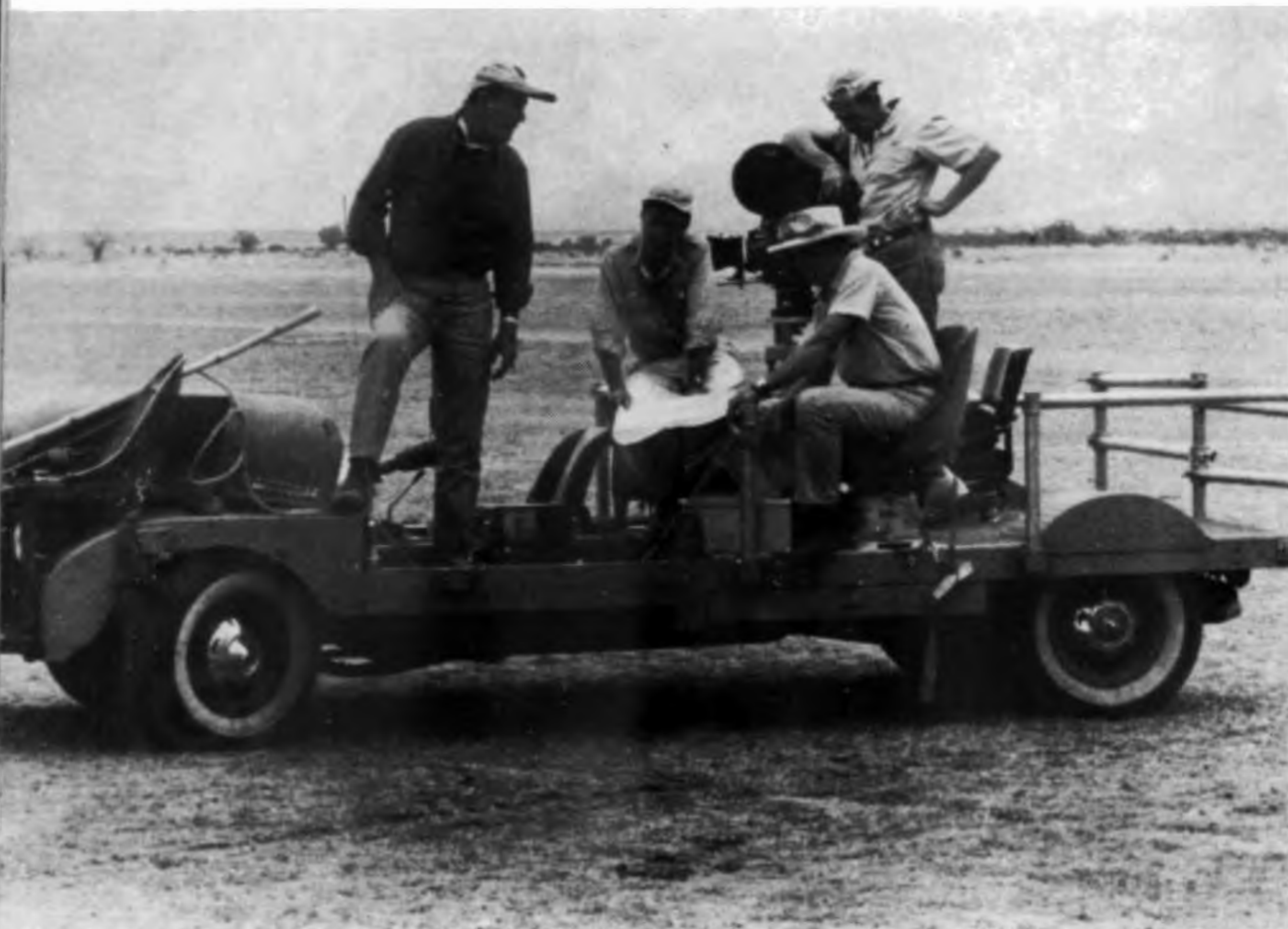
PLANNING THE ACTION —Strategy for upcoming action sequence is discussed by (from left) John Wayne, camera assistant Danny McCauley, director Howard Hawks, and cinematographer Russell Harlan. Camera car is modified Chevrolet chassis equipped with powerful motor and fitted with heavy aluminum guard plates.
