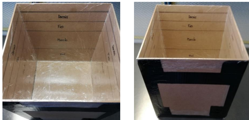
Figure 92: The mould used to cast the 2.4 GHz rhinoceros flank model.
