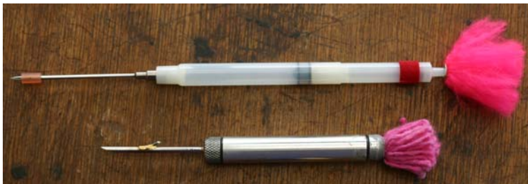
Plastic Daninject dart with 60mm smooth needle for boma work (top) and Cap-Chur dart with 50 mm barbed needle for field work (bottom).
