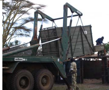
The Multilift system in Namibia (top) and the KWS “Hannibal” system in Kenya (bottom) are used to load/unload crates.
