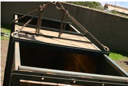
The front and back thirds of the crate roof are open to allow adequate ventilation.
