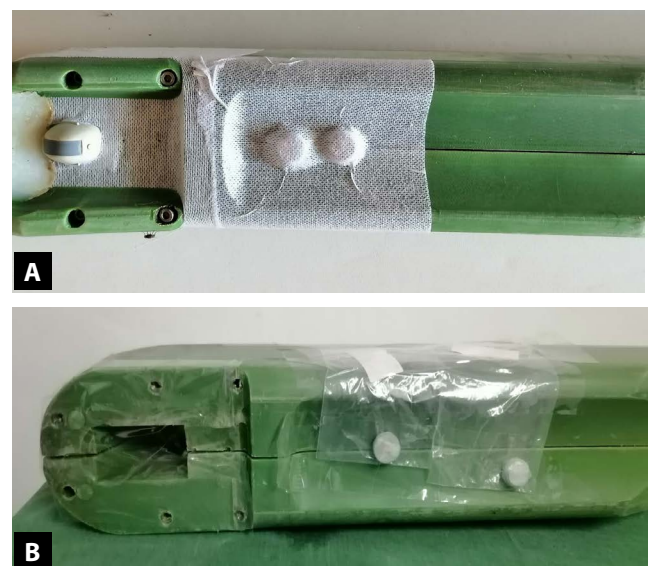
Figure 2: The iButtons were placed inside the PAP next to the aspiration line (A), and on the outside (B) of the PAP in order to record the temperature the oocytes will be exposed to and the rhinoceros' rectal temperature, respectively.
