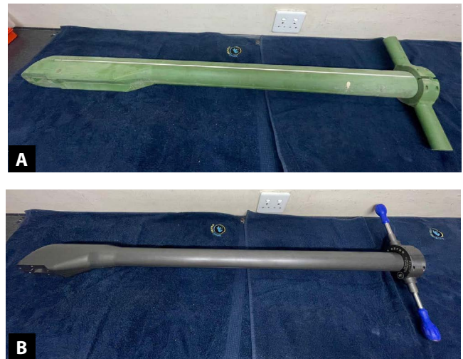
Figure 1: The aspiration probes used for rhinoceros oocyte pick-up in South Africa made from (A) polyvinyl chloride (143 x 11 x 10 cm, 11.3 kg) and (B) Aluminium (144 x 9,5 x 7.5 cm, 10.8 kg).
