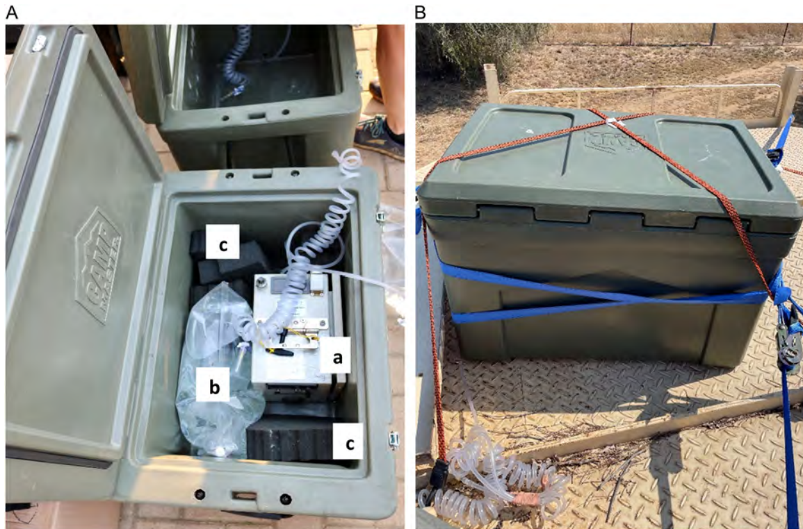
FIGURE 6 | (A and B) Infusion pump (a) along with one drip bag (b) and pieces of foam (c) for protection and positioning of the drip bags in the 60-L cooler box (A) and the cooler box strapped down on top of the rhinoceros crate (B). [Color figure can be viewed at wileyonlinelibrary.com ]
