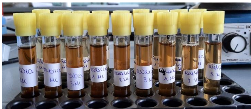
Figure 12: Sample tube containing 5 ml of supernatant after centrifugation
