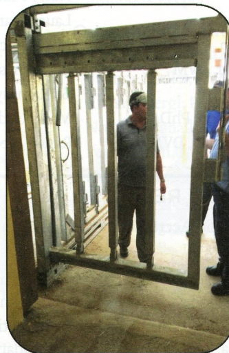
Meyer De Kock, Manager, inspecting the TAMER's® manual slide door with adjustable vertical pickets.
