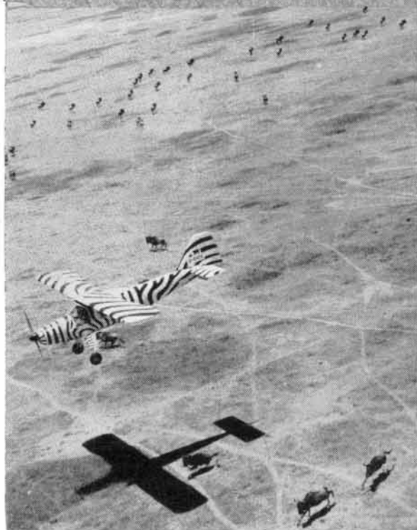
FIG. 1. The Dornier 27, used by the authors for the game census, was capable of extremely slow airspeed and landing on rough ground. The usual flying altitude was higher than shown here. Animals fled only short distances to both sides and remained in the counting strip. The lines on the ground are trails made by the animals.
