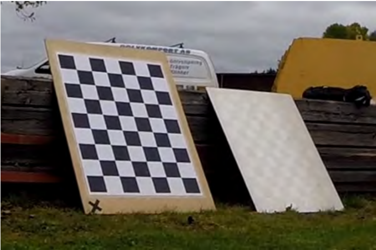
Figure 2.8: Two chess boards used for camera calibration. The left one is used for EO cameras while the right one is used for thermal cameras.
