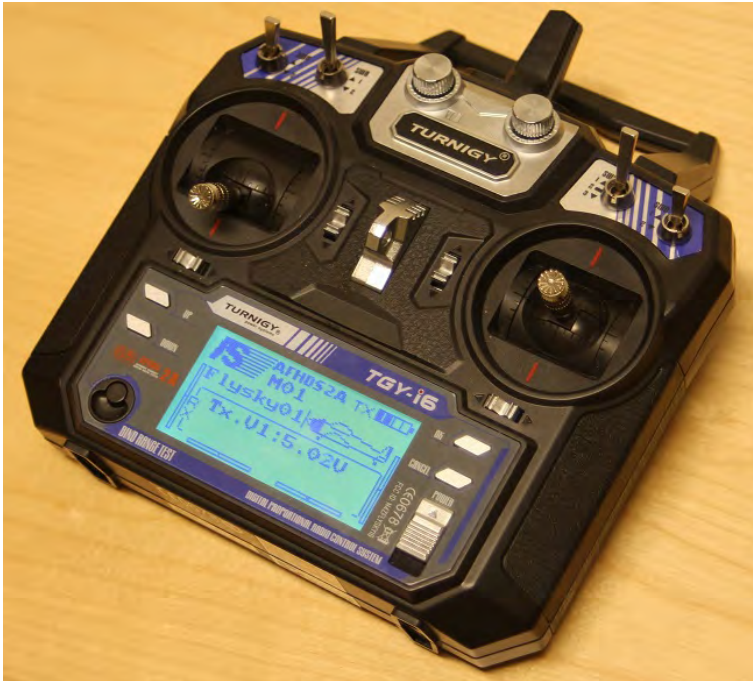
Figure 6.9: A typical remote control, with a radio transmitter, for aerial vehicles.
