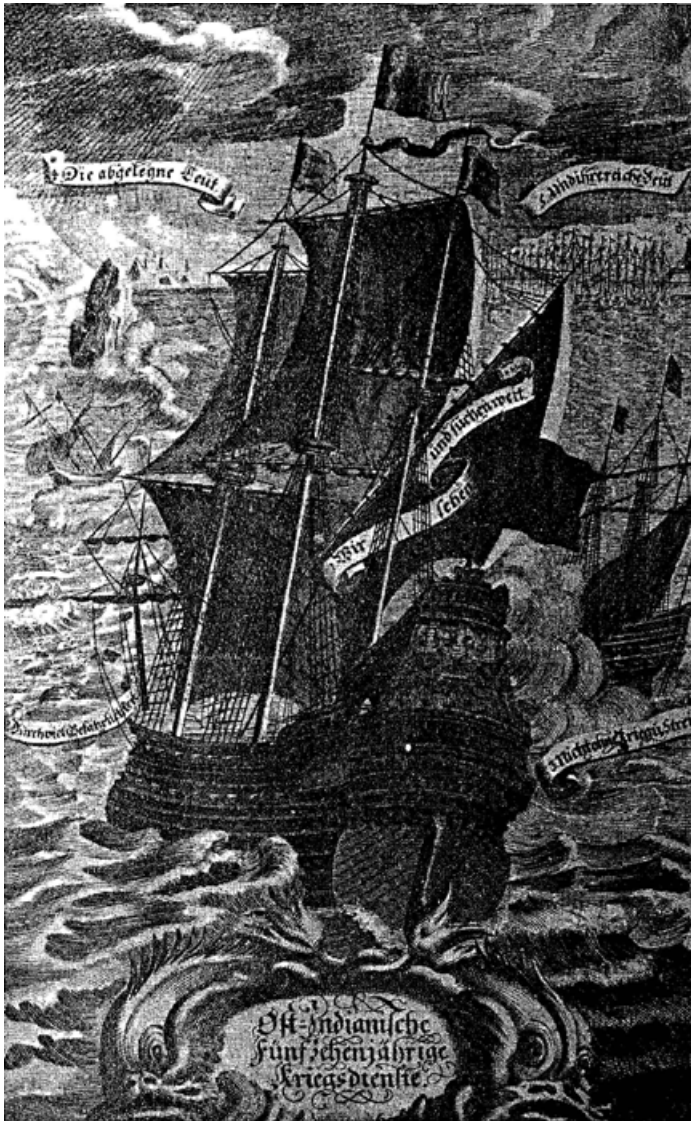
[14] Title page to item 10, Ost-Indianische funfzehnjährige Kriegsdienste , 'Fifteen years East-Indian Military Service.' The large flag at the maintop shows that the ship is Admiral. The rig is standard, with spritsail and spritsail-topsail furled, but the high
